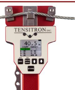
Precise, convenient cable tension measurement for MRO providers
